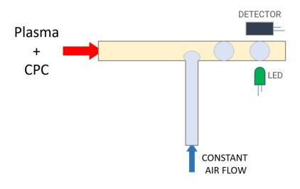
Figure 1. Basic structure of the device
