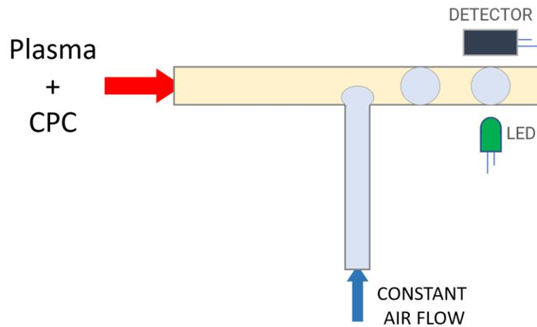
Figure 1. Basic structure of the device
